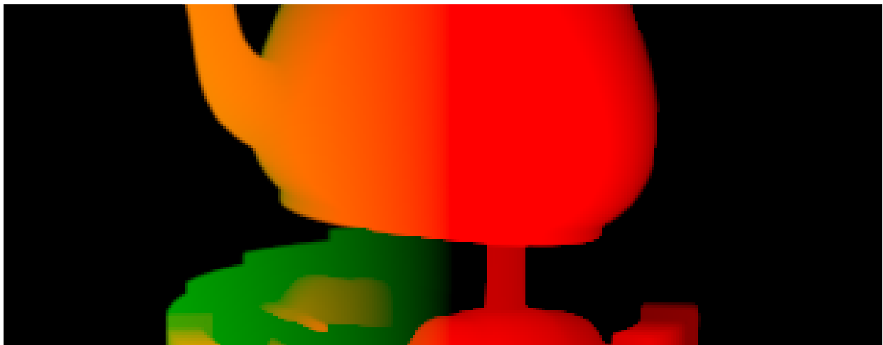
vector motionFore (Forward 2D raster-space motion vector)
