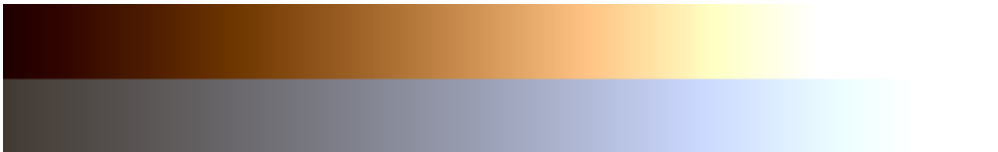
Top: linear ramp from 1,000K to 6,500K at -22 exposure. Bottom: linear ramp from 5,000K to 15,000K at -28 exposure.
