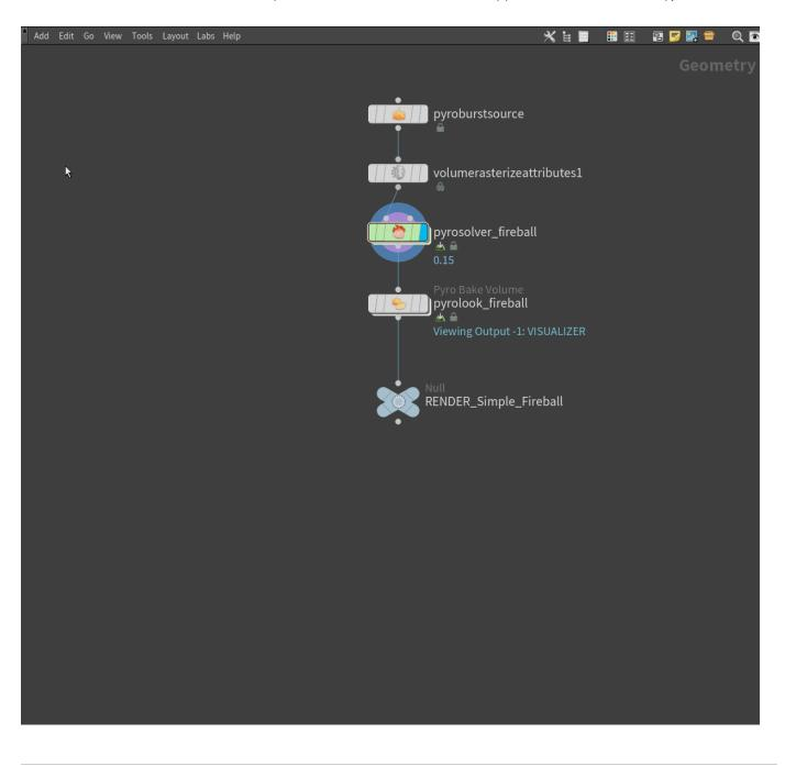
Once the network has been created, we need to drop down a RenderMan Kaboom Box node and pipe this into the network after the pyrosolver node.
