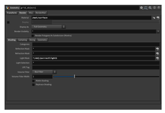
Below we omit the reflection of a sphere object as well as the light from the rect light.
