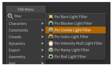
Parent the light filter OBJ to the light OBJ if you want the filter to inherit the transformation from the light.
