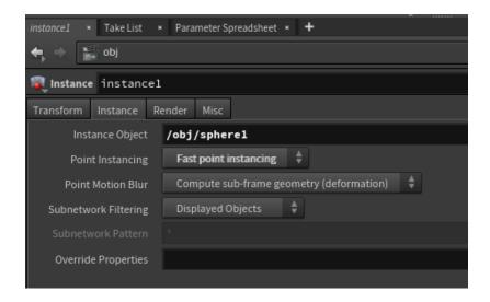
To override material for the instanced objects, we can use the Material SOP inside the Instance.
