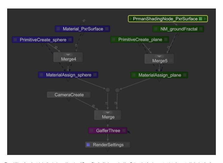
The addition of our fractal shading is done with series of PrmanShadingNodes, each with a Pattern that feeds an output into the next with the last feeding its result into **Color** input of the PxrSurface node:
