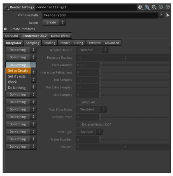
Integrator parameters are included in the RenderSettings (unlike their node representations outside of Solaris). The visible parameters are updated based on the selected integrator.
