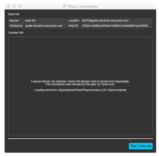
The LicenseApp is a useful tool for indicating the current state of your license server, it can be run on the client machines as well and will remotely query the server for the status.
