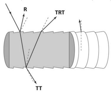
The Marschner specular model consists of three specular lobes using multiple specular transport paths shown above as directional arrows:
