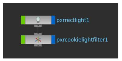
We can translate the light filter and scale it. It is best to translate the light filter in Z away from the light to avoid seeing the edge of the light filter.
