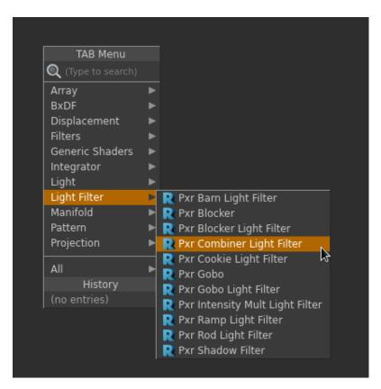
In the combiner, hit the + icon to dynamically create a light filter. Use the x icon to remove it. This combiner groups all the light filters under specific combining operators. That is, all the light filters under "Mult" will be multiplying by each others while "Max" will take the maximum of the light filters in the max group.
