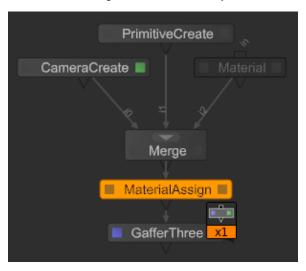
If you enable the MaterialAssign node for editing (hover over the node and hit **E**) you could also Shift+middle-click from the Material node into the **material Assign** box in the Parameter tab. Add the primitive to the Material CEL location in a similar manner to finish the material assignment:
