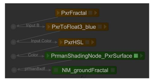
The above node graph uses the PxrFractal, PxrToFloat3 and PxrHSL patterns to convert fractal noise into a surface shader for our ground plane. Sunrise on a Sphere in a Fractal Sea:
