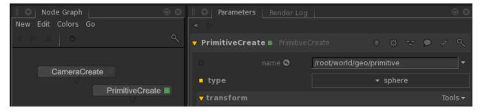
By default both the camera and the sphere will be created at the origin. Re-position either the camera and/or the sphere as needed so the sphere is in the camera's field of view. Use the Viewer tab to quickly look-through the camera and re-frame on the sphere or use the manipulators to move objects around in the Viewer.
