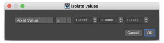
This simple command replaces with black any values that don't pass your test. You can compare the pixel value or luminance to a fixed value, using <, <=, ==, >= and >.
